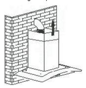
Measure the appropriate height and drill 2 x 8mm holes to accommodate the plate. Screw and tighten the upper wall with 2 screws provided.
